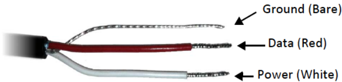
Figure 2: Pigtail End Wiring
