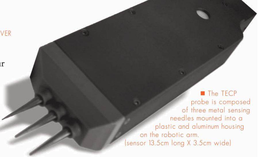
■ The TECP probe is composed of three metal sensing needles mounted into a plastic and aluminum housing on the robotic arm. (sensor 13.5cm long X 3.5cm wide)
