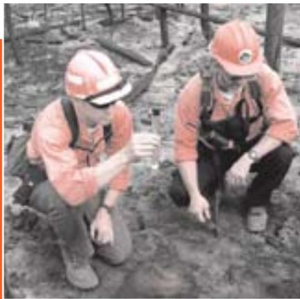
■ The Mini Disk Infiltrometer being used to identify water-repellent soil conditions after the Roberts Fire, Flathead National Forest.
