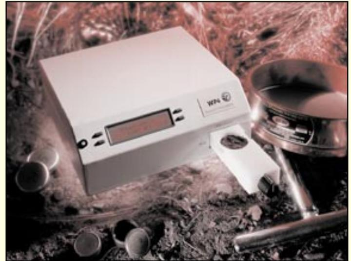
**WP4 Potentiometer measures water potential**—without waiting; a sample reading in under 5 minutes —without range limitations; 0 to -40 Mpa —without hassles; just load and read.
