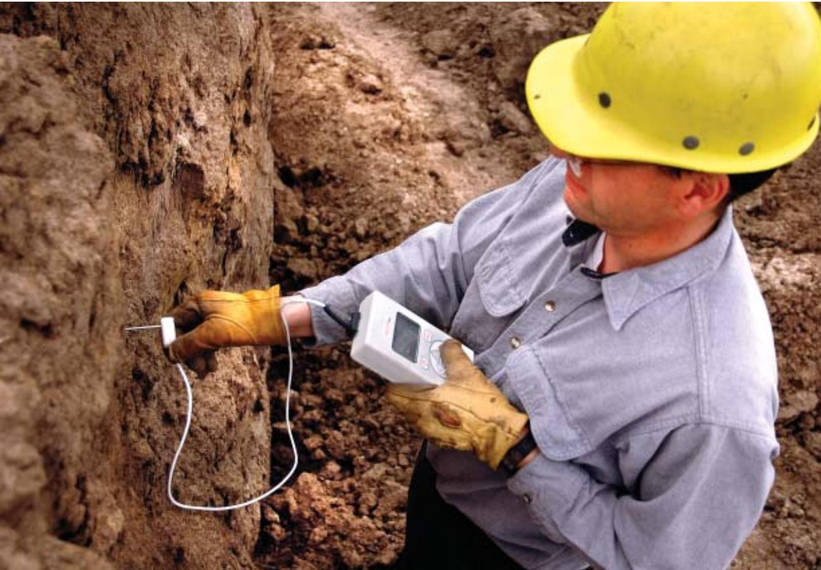
**The KD2 Pro with the TR-1 needle can accurately measure the thermal conductivity/resistivity of particles as large as coarse sand (1 mm diameter).**
