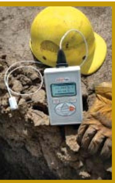
The KD2 Pro with the TR-1 needle can accurately measure the thermal conductivity/resistivity of particles as large as coarse sand (1 mm diameter). Larger materials can cause problems for
