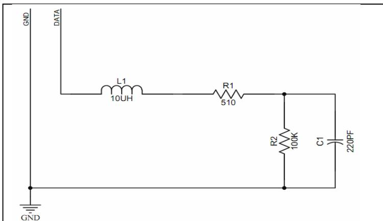
**NOTE:** This is a low impedance variant of the recommended SDI-12 Specification. This allows up to 62 sensors to be maintained on a bus.
