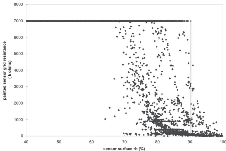
**Figure 1.** Grid resistance of a painted, baked resistance type leaf wetness sensor as a function of sensor surface relative humidity ( $rh_s$ ). Data were collected over a 60 day period in the summer and fall of 2005. Periods during and after rainfall and dew events were carefully removed from the data set, so any resistance less than the baseline level of 7000 k $\Omega$  are false liquid water events.
