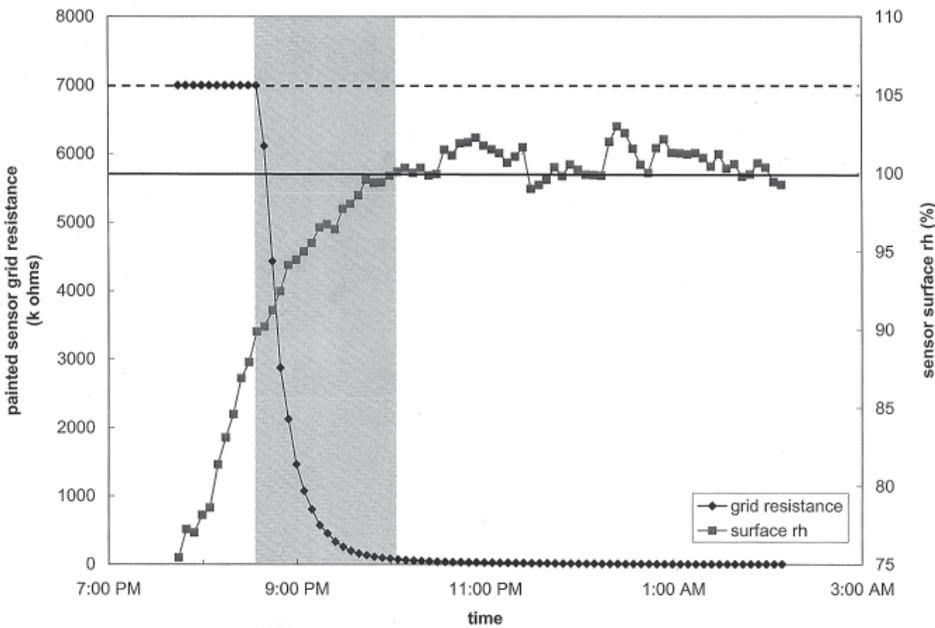
**Figure 2.** Grid resistance and surface relative humidity of a painted, baked resistance grid leaf wetness sensor over the onset of evening dew. The dashed horizontal line indicates the dry resistance of the sensor, with anything less than that threshold indicating surface wetness. The solid horizontal line indicates 100% rh<sub>s</sub> when dew will just begin to form on the sensor surface. The gray zone indicates the time duration when the sensor indicates liquid water, but none is present.
