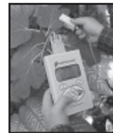
The new Leaf Porometer automatically measures stomatal conductance and eliminates human error by picking the end point. The direct
