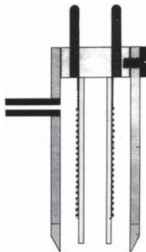
◀ Ellis Wallihan's porometer design with the Dunmore electronic humidity sensor (circa 1960.)
