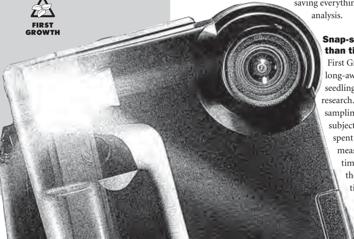
**FIRST GROWTH** MAKES GROUND COVER ANALYSIS simple with its digital camera made just for canopy cover research. First Growth identifies green plant tissue in every digital image. Custom software calculates the ratio of green pixels to total pixels. Image processing takes place inside the digital camera, so you get your readings right in the field.
