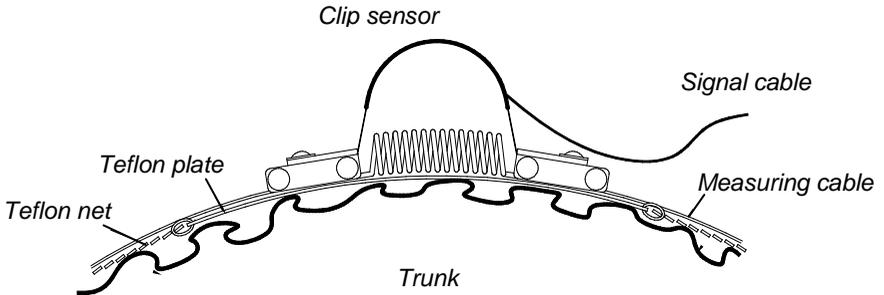
**Scheme of the installed D6**
