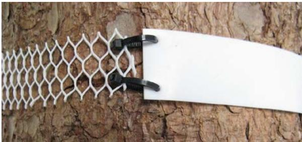
Lead cables ties trough the holes on the Teflon pad and connect it with one end of the Teflon net.
