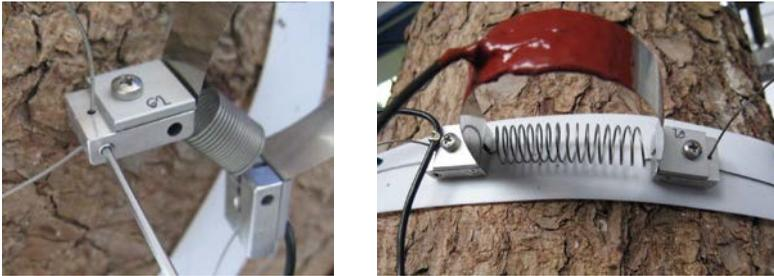
Lead the measuring steel cable around the trunk and cut it off with the required length. The length should be 5 cm longer than the circumference to allow a readjustment of the cable when the end of the measuring range is reached.
