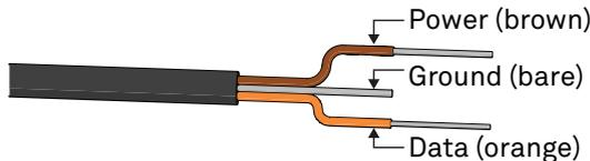
Figure 3 Pigtail wiring
