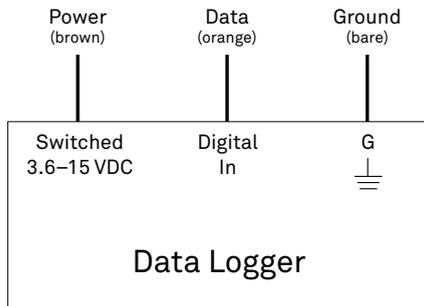
Figure 4 Wiring diagram
