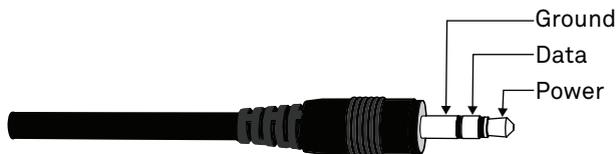
Figure 2 Stereo plug connector
