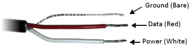
Figure 2: Pigtail End Wiring
