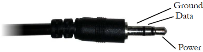
Figure 1: Stereo Connector
