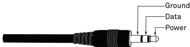
Figure 2 Stereo plug connector
