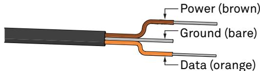
Figure 3 Pigtail wiring
