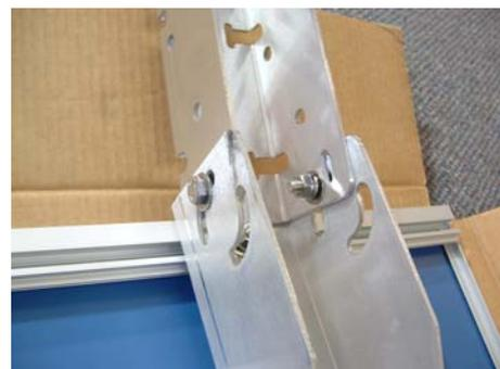
5) Attach the shorter bracket to the longer bracket by first aligning the lower holes and placing the bolts, washers, and nuts per the HPM 18/30 Mounting Kit Instructions.
