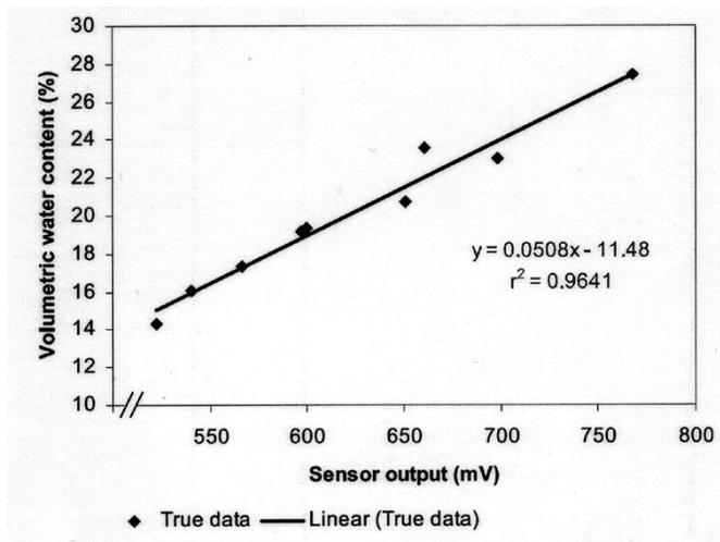
Figure 3. Regression between ECH20 Soil Moisture Probe readings and gravimetrically determined volumetric water content (%).
