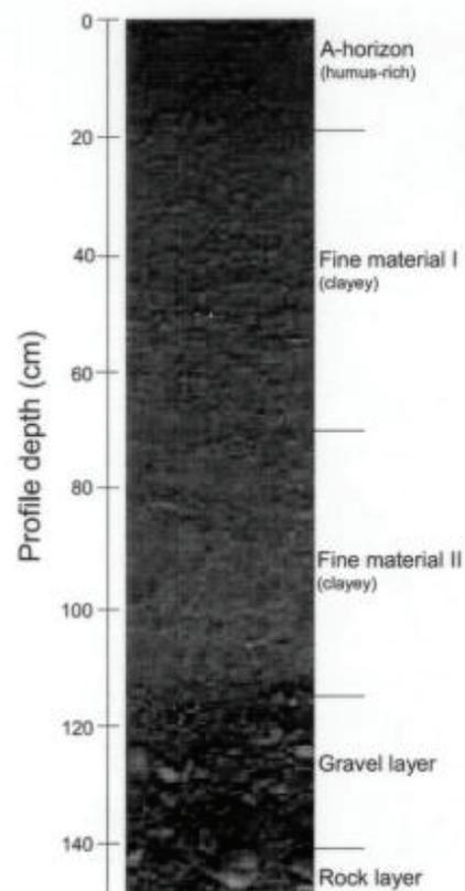
Figure 2. Soil profile of the experimental terrace site 30.
