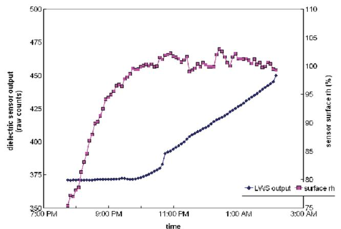
*Figure 3. Sensor output and surface relative humidity of an out-of-the-box dielectric leaf wetness sensor over the onset of evening dew. The dashed horizontal line indicates the dry baseline output of the sensor, with anything greater than that threshold indicating surface wetness. The solid horizontal line indicates 100% r<sub>h</sub>s when dew will just begin to form on the sensor surface. The gray zone indicates the time duration when the sensor indicates liquid water, but none is present.*
