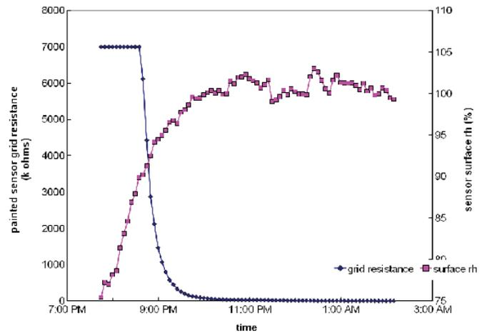
*Figure 2. Grid resistance and surface relative humidity of a painted, baked resistance grid leaf wetness sensor over the onset of evening dew. The dashed horizontal line indicates the dry resistance of the sensor, with anything less than that threshold indicating surface wetness. The solid horizontal line indicates 100% rhs when dew will just begin to form on the sensor surface. The gray zone indicates the time duration when the sensor indicates liquid water, but none is present.*
