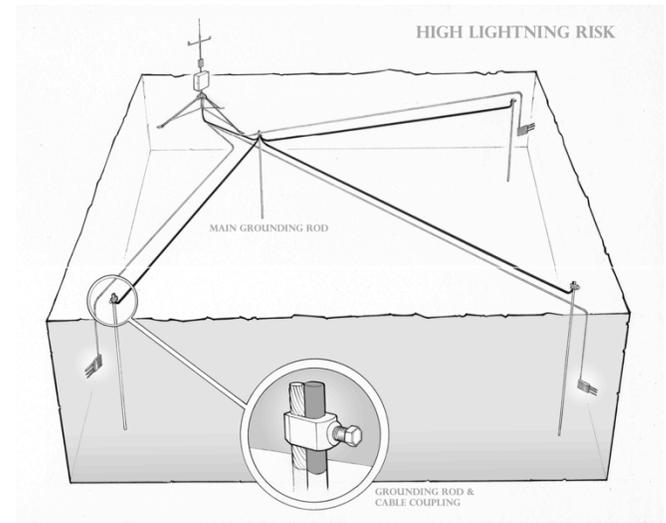
Figure 2. When lightning risk is high, ground rods may be required in the vicinity of each sensor location. As with the moderate lightning installation, #6 AWG copper wire connects each ground rod to the central rod, which is connected to the data logger.
