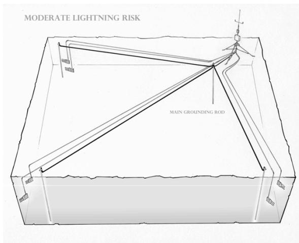
Figure 1. Ground rods in the general vicinity of groups of probes are connected back to a main grounding rod to which the logger is grounded. Ground rods should be driven 2 or more meters into the ground if possible and connected to the central ground through #6 AWG copper wire.
