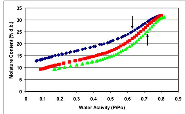
Figure 4. Moisture sorption isotherms of soft dog bits conducted at 15°C (♦), 25°C (■), and 40°C (▲).
