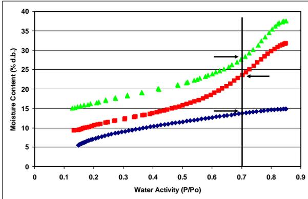
Figure 5. Moisture sorption isotherms for hard kibbles (◆), one type of soft bits (■), and another type of soft bits (▲). The line at 0.70  $a_w$  represents the natural water activity of the product.
