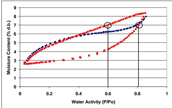
Figure 3. A working isotherm (♦) superimposed over a full isotherm curve (■) indicating that the working isotherm scans between the adsorption and desorption curves of the full isotherm. Also shown are the different water activities associated with 7% moisture depending on if the product is wetted or dried.
