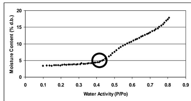
Figure 6. Moisture sorption isotherm for spray dried milk powder showing a phase change occurring at a critical water activity of 0.43.
