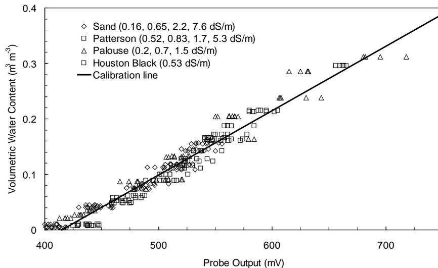
Figure 1. Calibration data for five water content sensors running at 70 MHz in four mineral soils over a range of electrical conductivities (shown in parenthesis).
